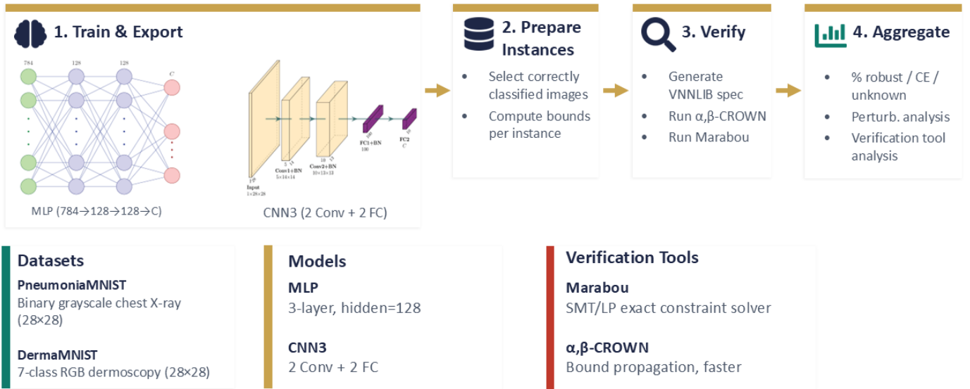
Fig. 2: Overview of the verification pipeline. A trained model, perturbation set, and formal specification are combined to produce per-instance verification outcomes using multiple tools.
